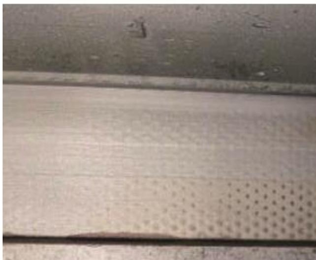
Fig. 5. Residual of a brazed joint after removing the honeycomb seal
