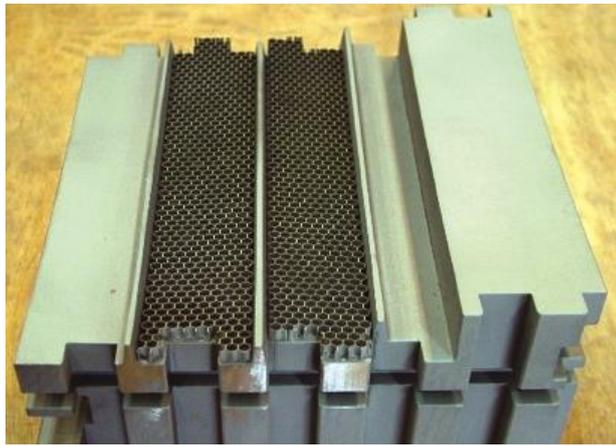
Fig. 1. Gas turbine second stage rotor blade shroud MS6001
