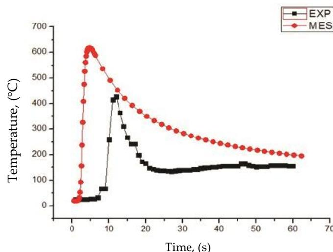
**Fig. 14.** Comparison of thermal cycles obtained by the finite element method (FEM) and experimentally (EXP) for a point 10 mm away from the weld axis
