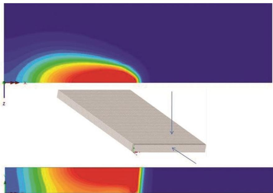
**Fig. 10.** Temperature field during the plasma-MAG hybrid welding process (top view and in longitudinal section)
