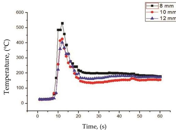
**Fig. 13.** The thermal cycle obtained during the experimental tests of plasma-MAG hybrid welding recorded for points located 8, 10 and 12 mm from the weld axis
