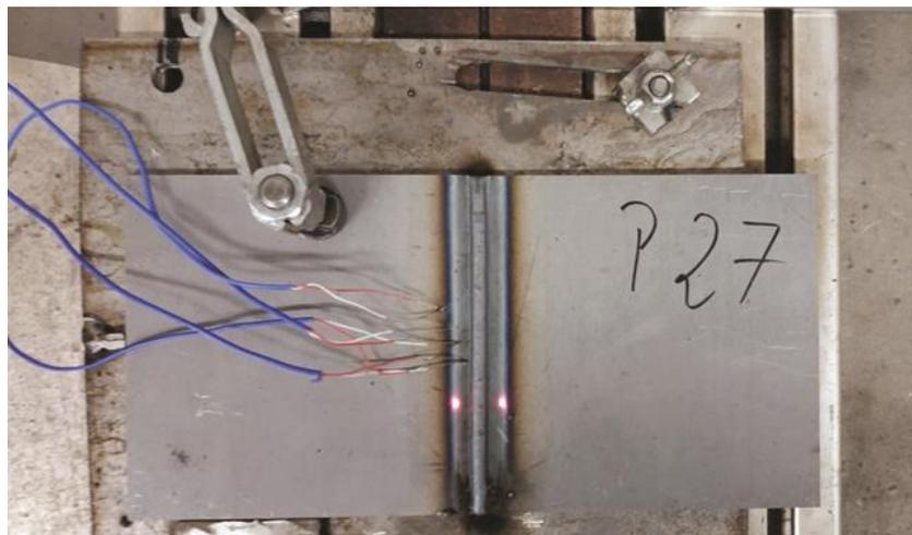
**Fig. 5.** View of the thermocouples attached to the test sheet after the MAG butt welding test
