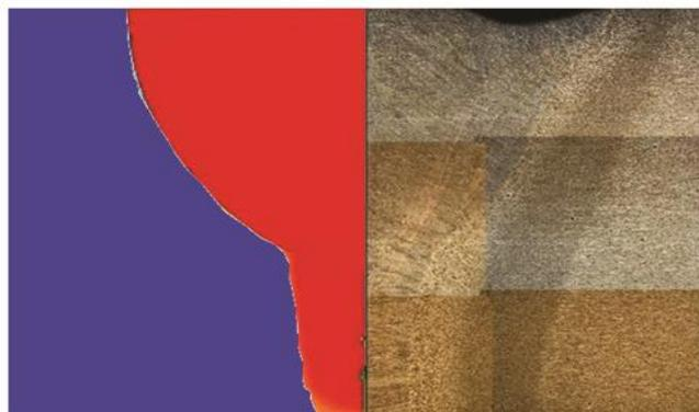
**Fig. 12.** Comparison of the weld shape in the cross-section of the hybrid-welded joint according to the results of the temperature distribution (left) and the metallographic tests of the weld (right)
