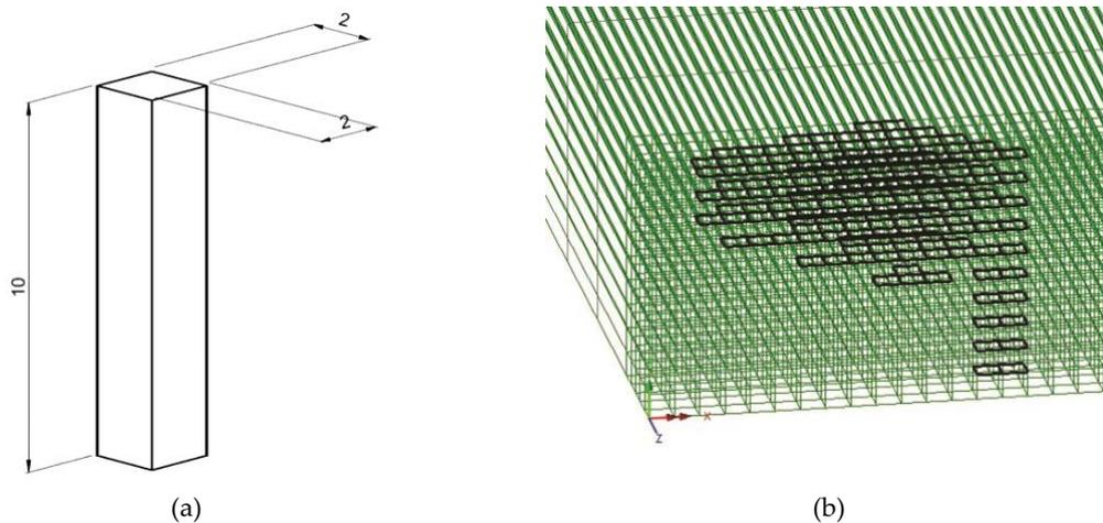
**Fig. 9.** The heat source model adopted for the plasma part of the hybrid welding process (a) and the graphic representation of the entire hybrid heat source model against the background of the finite element mesh (b)
