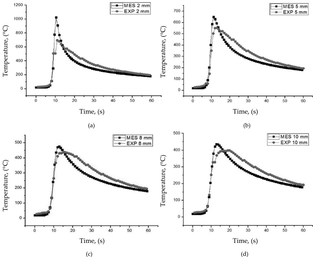
**Fig. 8.** Comparison of thermal cycles obtained from modeling with the finite element method (FEM) and measurements with thermocouples (EXP) for measuring points at different distances from the weld axis: a) 2 mm, b) 5 mm, c) 8 mm, d) 10 mm
