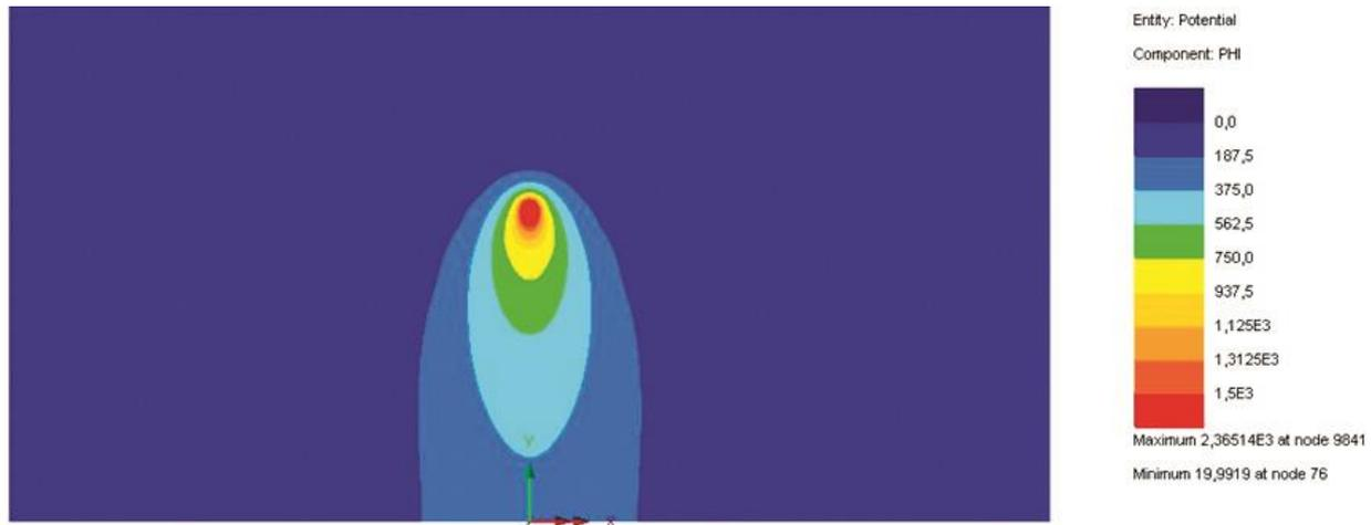
**Fig. 2.** The temperature field at the selected moment of time for the Goldak model determined for the MAG butt welding of plates
