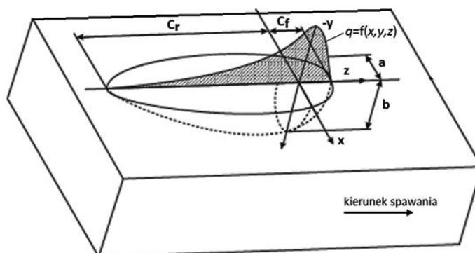
Fig. 1. Geometric parameters described by the double ellipsoidal model of the welding heat source according to Goldak
