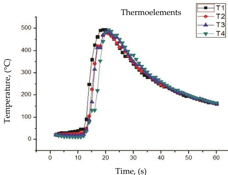
**Fig. 7.** Thermal cycle recorded by four thermocouples mounted 5 mm from the weld axis
