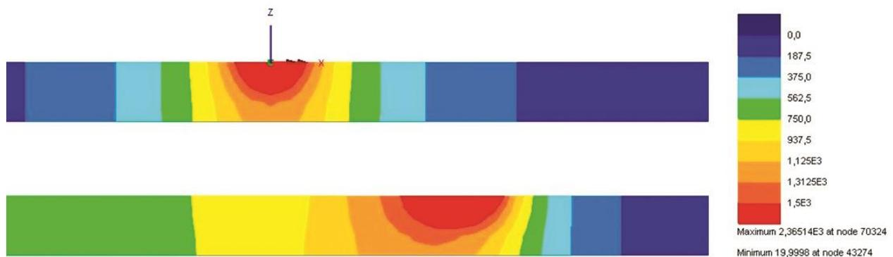
**Fig. 3.** Temperature distribution in the cross-section of the joint (top) and in the longitudinal section (bottom) for the Goldak model when welding sheets with the MAG method
