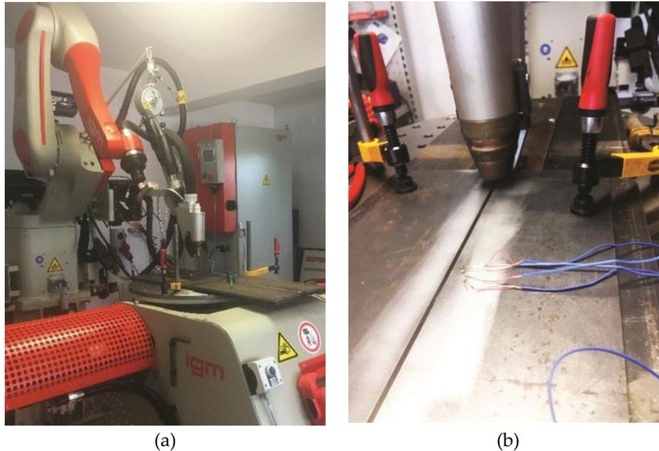
**Fig. 11.** Stand for experimental tests of the plasma-MAG hybrid welding process with temperature registration using thermocouples: a) hybrid welding station with a KUKA KR 16-2f robot, b) welded joint with fixed thermocouples
