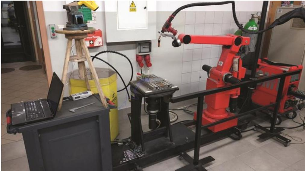
**Fig. 4.** Robotized station for MAG welding
