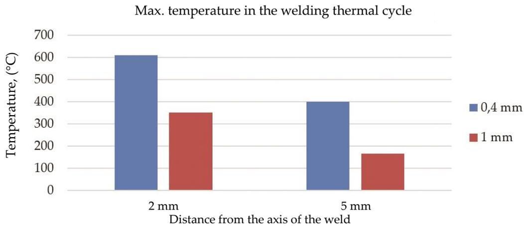
**Fig. 6.** Graphs of the dependence between the diameter of the thermocouple (0.4 and 1 mm) and the maximum recorded temperature in the welding cycle
