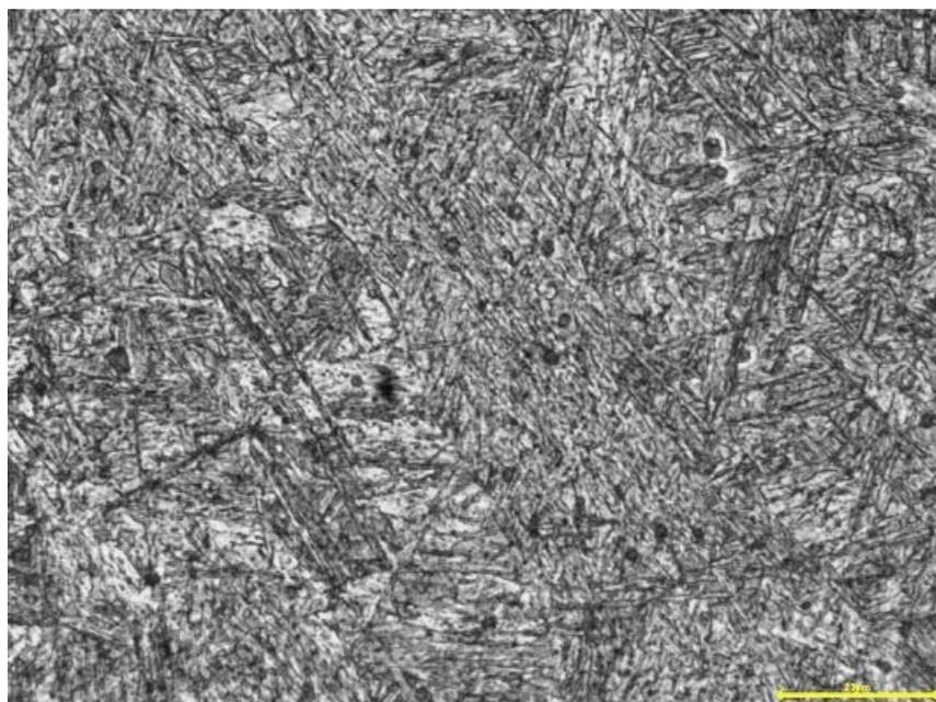
**Fig. 2.** Weld structure made using the Union X96 electrode wire
