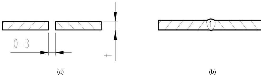
Fig. 1. a) Shape of the groove; b) welding method
