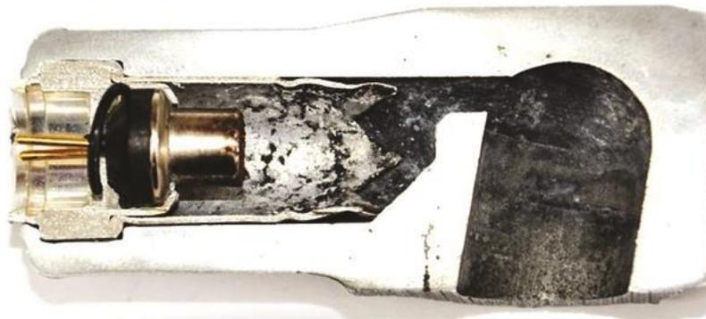
**Fig. 3.** The method of securing the pyrotechnic charge in a cast housing
